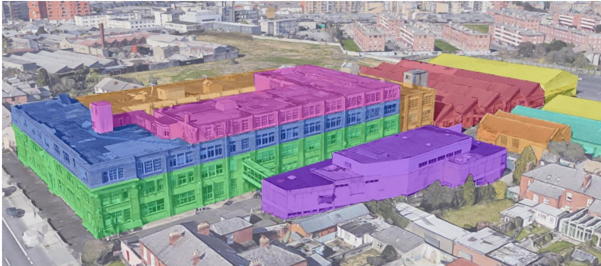
FIGURE 14.13: OVERLAY ON AERIAL IMAGE FROM GOOGLE MAPS, SHOWING THE PHASED DEVELOPMENT OF THE EXISTING SITE OF THE FORMER PLAYER WILLS FACTORY.
